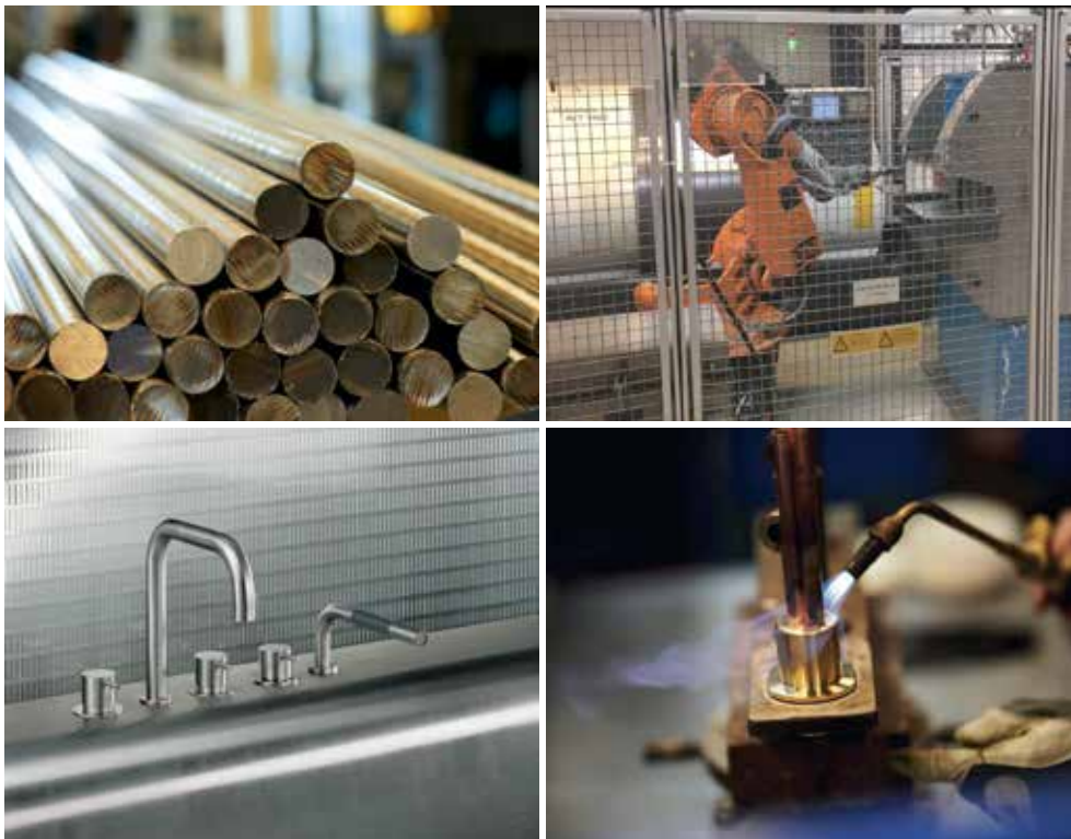
Figure 13. VOLA. From upper left clockwise: raw material (brass cylindrical bars), robot manufacturing, human interventions, finishes and touches, and finished product.
