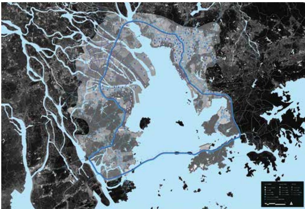
Figure 1. A masterplan of the Pearl River Delta Special Ecological Area depicts the water supply loop connecting various resources distributed throughout the various political entities of China's Pearl River Delta.
