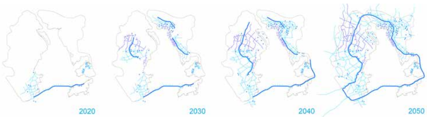
Figure 10. A phasing diagram of how the Pearl River Delta Special Ecological Area water resource loop may be developed over the coming decades.
