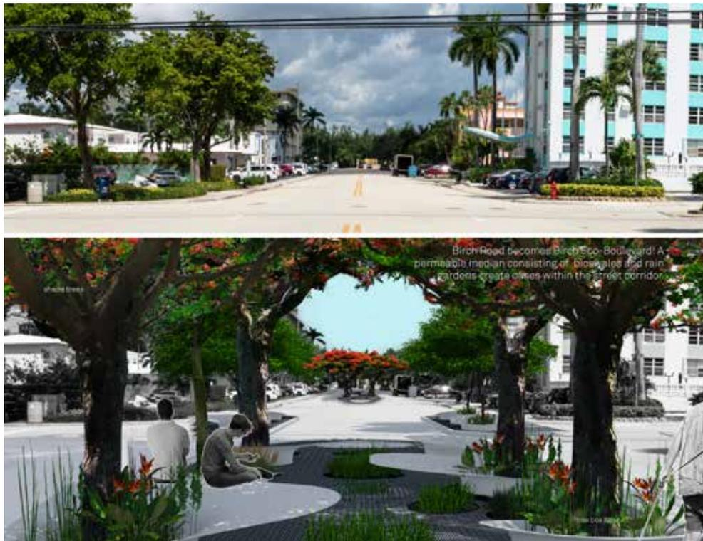
Figure 10. Before and after of street retrofit illustrating rain gardens and bioswales that act as “biopumps.”
