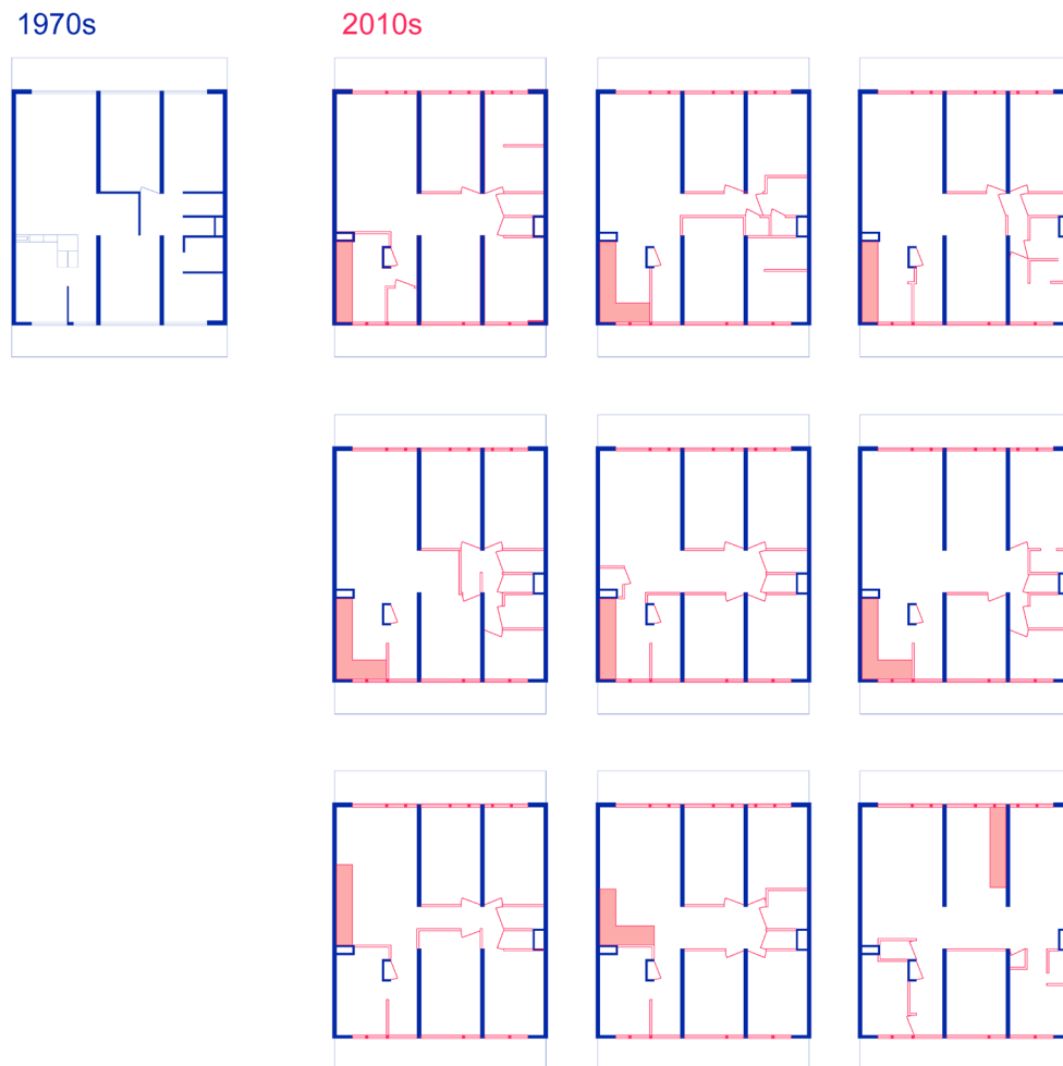
Figure 15. An example of the de-standardization of housing. On the left, the standard three-room apartment delivered in the 1970s; on the right, some examples of the different configurations adopted during the renovation. The permanent structure is in blue, the variations in red.
