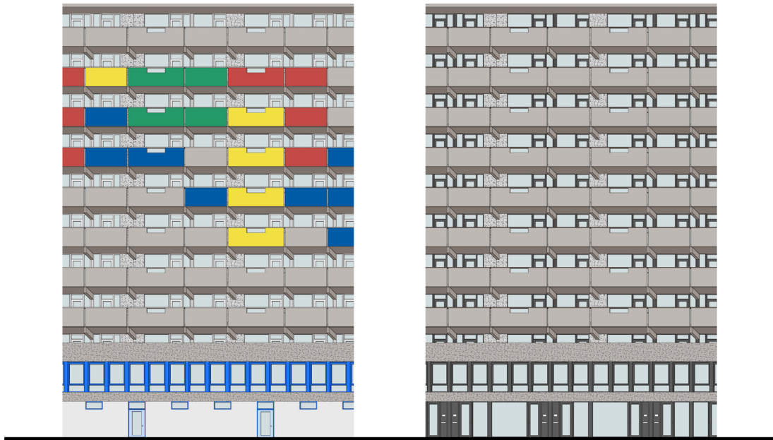
Figure 16. Bijlmermeer/Kleiburg. Portion of the elevation in axonometry. Comparison of original design (left) and renovation (right).
