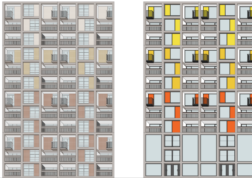
Figure 4. Park Hill/Phase one. Portion of the elevation in axonometry. Comparison of original design (left) and design realised in phase one (right).
